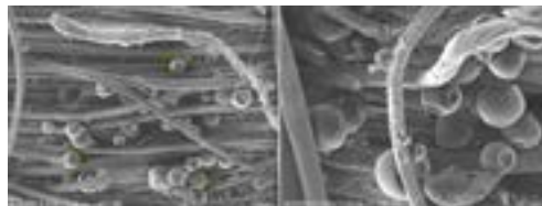
Figure 5. Microcapsules on black patterned fabric at 400x and 1000x magnifications. Source: The Researcher
